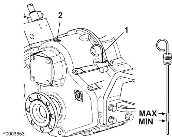
**Check the oil level in the reverse gear**
