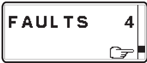
Faults are stored and malfunctions have been registered
